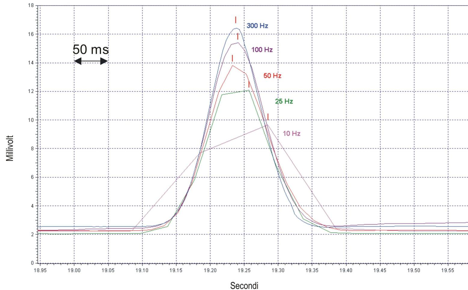
**Figure 1** - Effect of the acquisition frequency on the peak shape. In FAST-GC, peaks could have very narrow width (even less than 500ms). For this reason is important to have an "high-speed" detector able to collect at least 10 points for every peak, thus to correctly describe the peak itself. In this way the peak can be properly integrated and quantified. **In FAST-GC an acquisition rate of at least 50Hz is recommended.**
